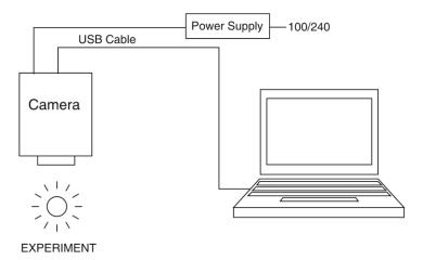
Figure 2. Typical Imaging Experiment Layout (Air-cooled Camera)
